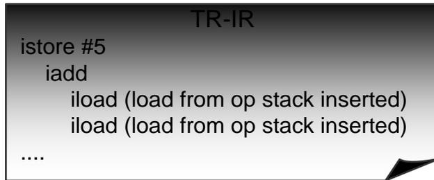
IL gen translates the trace into TR-IR. Implicit loads are inserted before the first bytecode if the operand stack is not empty upon entry to the trace.
