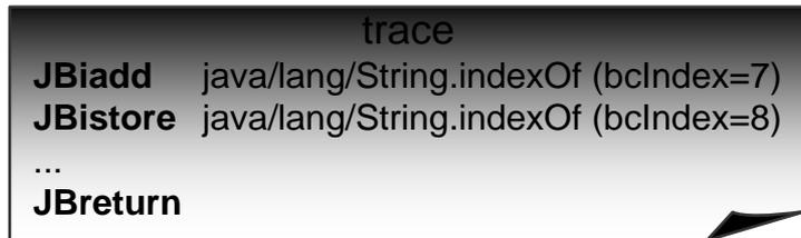
trace selection engine forms a trace. each BC is labeled by the method name and bcIndex to show its origin. *(starting from JBiadd is not possible in Java method compilation!)*
