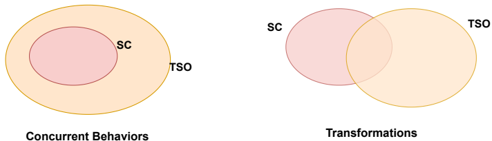
Figure: The final relation between SC and TSO w.r.t. permitted concurrent behaviors (left) and optimizations (right)
